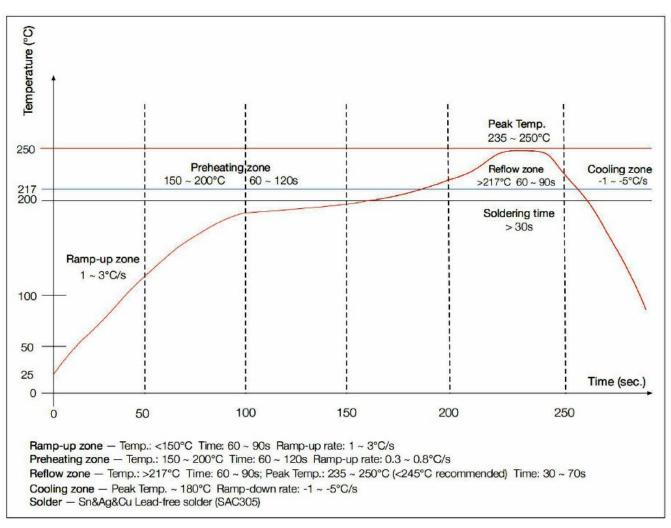
The module Must go through 100  $^\circ\!\!\!\!{}^\circ\!\!\!{}^\circ$  baking for at least 12 hours before SMT AND IR reflow process!
